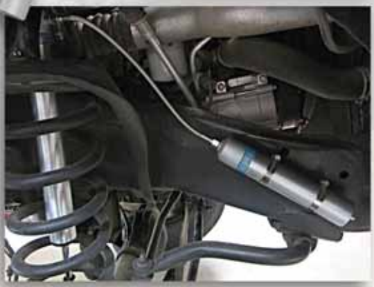
Some applications require the reservoir to be mounted to the frame of the vehicle
