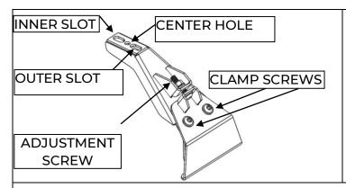
4. Prepare the mounts for installation by loosening the Clamp Screws (2 per mount) and the Adjustment Screw (1 per mount) so that the mount will open enough to fit over the rain gutter of the vehicle. in some cases the mounts may need to be partially disassembled in order to fit the mount clamp over the rain gutter. (If all mounts are not assembled, assemble them to match the sample.)
