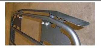
3. Position Air Dam so that there is a constant gap size between the Air Dam skin and the leading tube of the platform rack (figure 13). Fully tighten all hardware once you are happy with the position/gap. (This gap will provide clearance at the front tube for ropes, straps, and hooks to secure your load. The gap will be approximately 3/4" with the Air Dam positioned completely forward in the mounting slots.)
