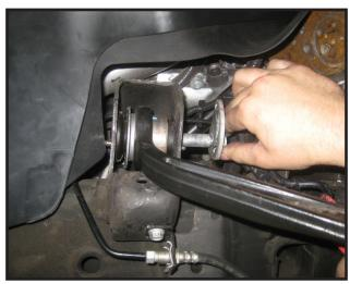
6. Remove the OE upper control arm from the vehicle.
