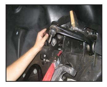
5. Remove the cam adjusting bolts that hold the upper control arm to its frame mounts. **Take note of the location of these bolts.**
