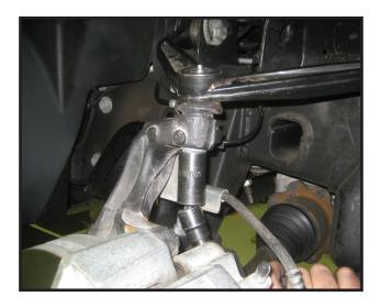
4. Carefully seperate the upper ball joint from the steering knuckle by using a hammer to strike the knuckle and breaking it loose.
