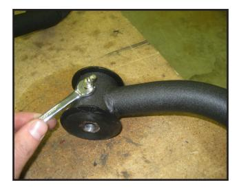
11. Install the new upper control arms into the vehicle using the OE cam adjusting bolts and hardware. Make sure to install the bolts in the same orientation they were removed. **Torque to 125 ft lbs.**
