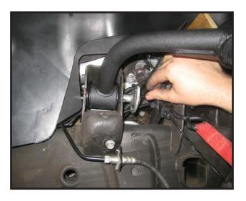
12. Carefully raise up on the lower control arm so that you can install the new upper ball joint into the steering knuckle. Secure using the new castle nut and cotter pin. If you are not able to install the cotter pin because the hole in the ball joint does not line up with the castle nut, DO NOT loosen the nut, but instead, tighten it until the cotter pin can be installed. Torque to 70 ft lbs.
