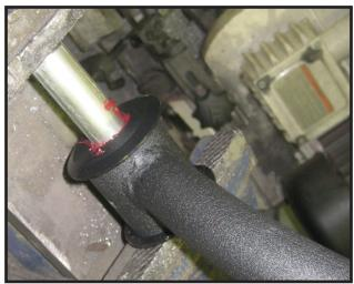
10. Install the threaded grease fittings into each eyelet, be sure to not over tighten these. Also make sure to point them towards the outside of the vehicle to allow for easy access.
