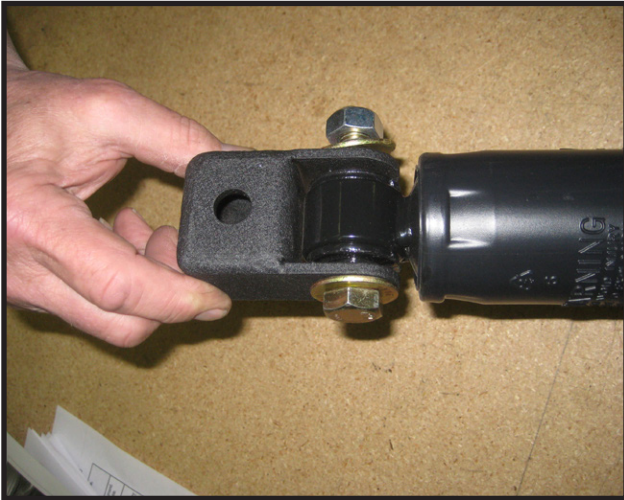
42. Re-install the rear shocks using the OE hardware
