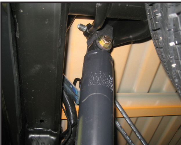
42. Re-install the rear shocks using the OE hardware
