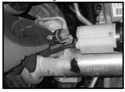
13. Carefully remove the front drive line from the front differential. Save the hardware. Carefully tie the front drive line up and out of the way.
