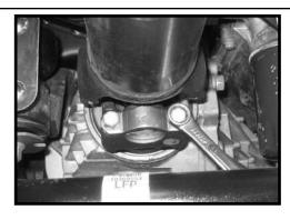
14. Working on the driver side, remove the CV axle from the front differential flange. Save the hardware. Special note: Take special care not to over extend the CV axle during removal. Rest the CV axle on the lower control arm. Repeat procedure on the passenger side.
