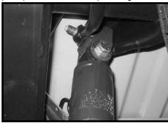
axle. Carefully raise up on the hydraulic floor jack until the Working on the driver side, zip tie the ABS line to the OE coil springs seats properly into the vehicle. Repeat proce-bump stop bracket. Repeat procedure on the passenger side.
