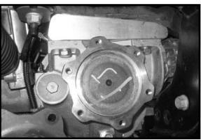
25. Locate (4) 12 mm x 35 mm bolts from hardware bag 14056NB1. Also, locate (2) 12 mm lock washers and (2) 12 mm fender washers from hardware bag 14056NB3. Secure the passenger side of the differential to the newly installed passenger side differential spacer using the new hardware. Make sure to use loctite and torque to **55 ft lbs**.
