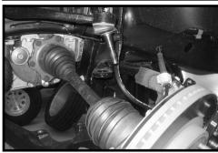
11. Working on the driver side, remove the upper control arm from the upper control arm location. The upper control arm may be discarded but save the upper control arm hardware. Repeat procedure on the passenger side.
