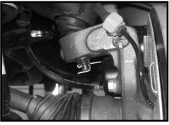
39. Working on the driver side, re-install the CV axle to the front differential using the OE hardware. Make sure to use loctite and torque to 45 ft lbs. Repeat procedure on the pas-
