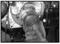
harness from the front differential. Tie the 4WD wiring harness up and out of the way. **Special note: Take special** ber from the OE location. Save the cross member and hard-care not to kink the wiring.
