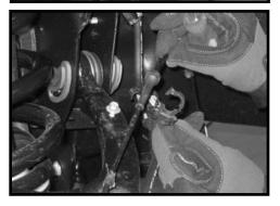
5. Working on the driver side, remove the sway bar end link from the sway bar and lower control arm. Save the end link and hardware. Repeat procedure on the passenger side.
