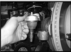
7. Working on the driver side, remove the lower hardware securing the strut to the lower control arm. The hardware may be discarded. Repeat procedure on the passenger side.
