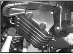
45. Working on the driver side, center and torque the OE cam bolts to 95 ft lbs. Repeat procedure on the passenger side.
