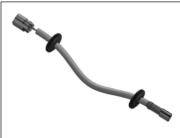
(Fig 7) Slide (2) Rubber Grommets onto OE Wire Harness
