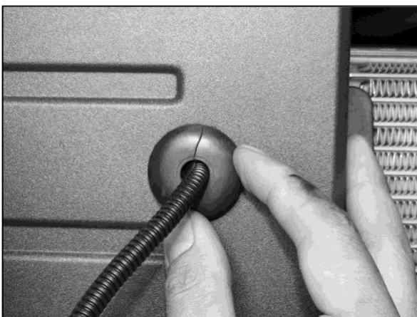
(Fig 12) Push Rubber Grommet on Harness into sensor hole (Bumper used for Example Only)
