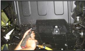
3. Carefully disconnect all (3) electric wiring harnesses from the rack and pinion.
