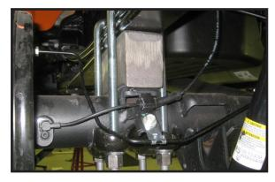
47. Locate the new rear shock relocation brackets. Locate (2) 9/16" x 3" bolt, (4) 1/2" USS flat washers and (2) 9/16" unitorque nuts from hardware bag 14059NB. Install the new shock relocation brackets to the top of the stock shocks 44. Locate (2) new 3" lifted blocks. Working on the driver and secure using the new hardware. Do not tighten at this
