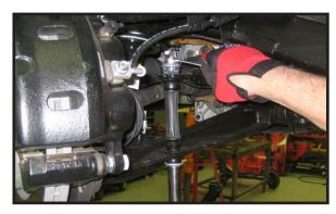
a hammer and striking the knuckle will help break the strut aside. Repeat procedure on the passenger side. taper. Take special care not to damage the outer tie rod dust boot during removal. Repeat procedure on the passenger side.
