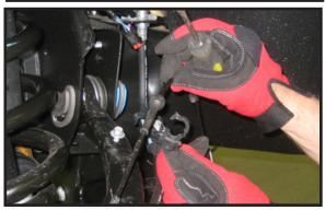
from the sway bar and lower control arm. Save the end link and hardware. Repeat procedure on the passenger side.
