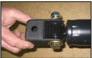
the upper and lower location using the OE hardware. Make the vehicle. sure to use loctite and torque to 85 ft lbs. Move back to the new 9/16" hardware and add some loctite and torque to 85 This Suspension System comes with (1) installation ft lbs. Repeat procedure on the passenger side.
