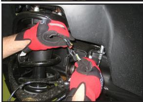
13. Working on the driver side, remove the ABS line from the OE upper control arm. The hardware maybe discarded
