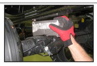
45. Carefully raise up on both hydraulic floor jacks at the same time until the spring assembly sits flush with the newly installed 3" lifted block.
