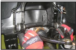
21. Locate the new upper control arms. Locate (8) poly bushings and (4) sleeves from hardware bag 14059PL. Install the new bushings and sleeves into the new upper control arms. Special note: Make sure to use a fair amount of lithium or moly base grease before installing the new bushings and sleeves into the control arms. This will increase the life of the bushing as well as help prevent squeaking.
