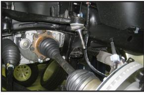
20. Working on the driver side, remove the upper control arm from the upper control arm location. The upper control arm may be discarded but save the upper control arm hardware. Repeat procedure on the passenger side.
