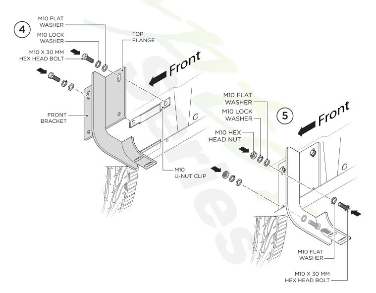
7. Attach the Step Bar to each Bracket using two (2) M10 x
