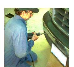
Step 3: Align grille guard to truck and mark holes. Drill 1/2 inch holes (2 per side) through chrome bumper and bumper support bracket (installed in step 2).
