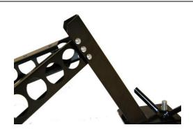
3. Locate the upper leg support plate (A). This will bolt onto the top of the support legs using four of the 1" Allen head bolts and lock nuts. Make sure when you install it that the bent tab at the top points up. Again, leave bolts loose until final assembly.
