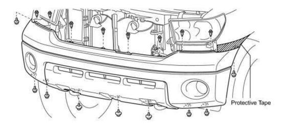
5. If your vehicle has Fog Lights, Disconnect the wire attachments and Detach the 4 claws to remove the bumper cover.
