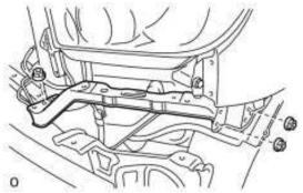
9. Remove Front Bumper Reinforcement
