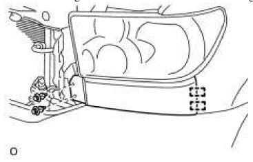
2. Remove Front Bumper Cover underneath each wheel well.
