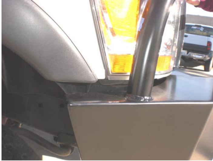
Figure 3: Correct body gap with new bumper installed
