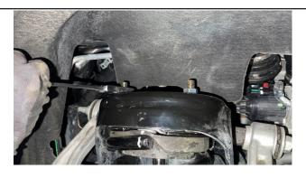
15. Tighten all 4 lower control arm Cam bolt hardware. **Torque to 130 ft lbs.**
