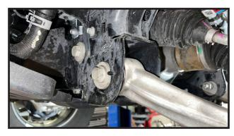
12. Re-install sway bar on to the lower control arms and to the the frame mounts. **Torque bolts to 75 ft lbs**.
