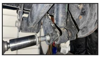
23. Install remaining 3/8" flange nuts on the upper strut mount. Repeat on passenger side. Torque to 55 ft lbs.
