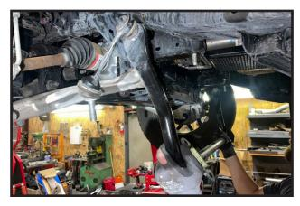
Remove the lower strut mounting hardware on the driver and passenger side.
