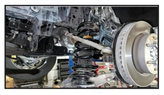
Remove the guide pin from the strut top hat. Looking at where the coil spring ends mark a line on the spring, Isolater and top hat, on the center of the 2 studs.
