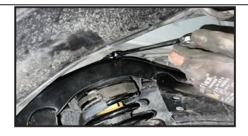
24. Re-install inner fender well clips. repeat on passenger side.
