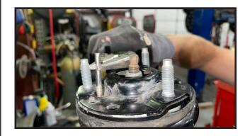
20. Locate part # 22500-01, Install on top of the rear sruts using OE hardware. **Torque nuts to 85 ft lbs**
