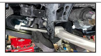
Remove lower control arms from mounting pockets and lower strut mounts. Remove the remaining nut on the top strut mount and remove struts.
