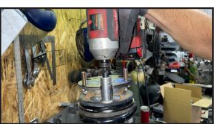
10. locate the 3/8" flange nuts. Re-install strut into the upper mount. use one of the 3/8" flange nuts to hang the strut loosely . Repeat on passenger side
