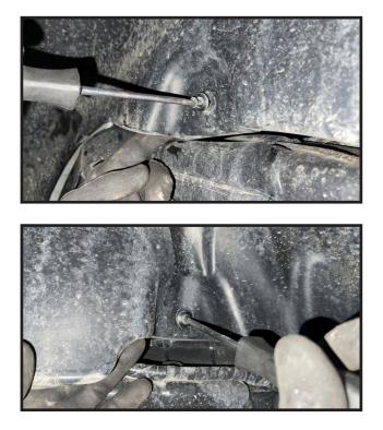
17. Remove the track bar mounting bolt on the axle side.
