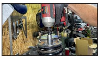
21. locate the 3/8" flange nuts. Re-install strut into the upper mount. use one of the 3/8" flange nuts to hang the strut loosely. Repeat on passenger side
