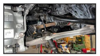
5 . Remove lower control arm cam bolt hardware on the driver and passenger side.
