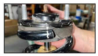
8. Using a strut spring compressor, Remove the nut on the top hat. Remove the top hat only and rotate 180 degrees, so there is now lined up to the mark on the coil spring and isolater. Re compress spring and re-install nut, **Torque to 80 ft lbs.**
