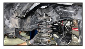
19. Remove the guide pin from the strut top hat.
