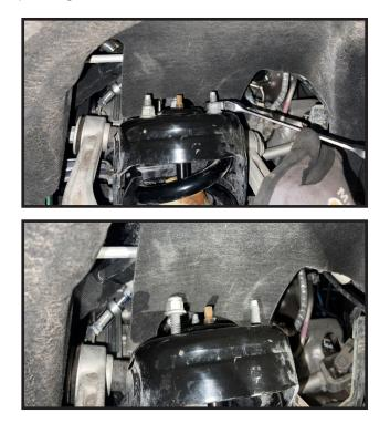
Remove the lower sway bar endlink hardware on the driver and passenger lower control arms. Remove the hardware securing the sway bar to the frame and remove the sway bar.
