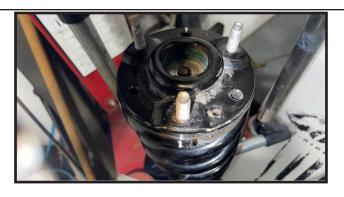
9. Locate part # 22500-01, Install on top of the front sruts using OE hardware. **Torque nuts to 85 ft lbs**
