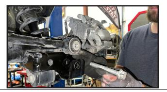
Remove the 3 upper strut mounting nuts, Remove the lower strut mounting hardware and remove the strut. Repeat on passenger side.
