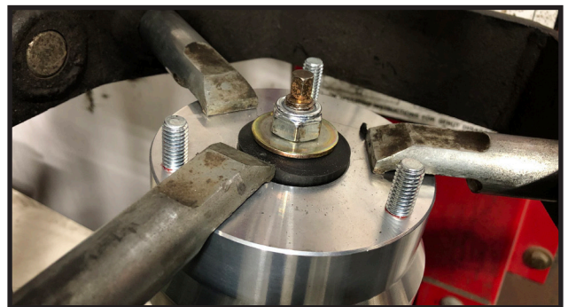
19. Locate part # M22706 poly bushing, S10305 washer and M12NLN 12 MM nylock nut. install them onto the shock stud. Tighten tell nut bottoms out.
