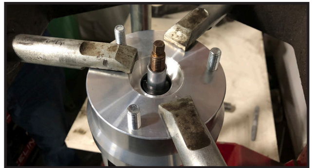
19. Locate part # M22706 poly bushing, S10305 washer and M12NLN 12 MM nylock nut. install them onto the shock stud. Tighten tell nut bottoms out.
