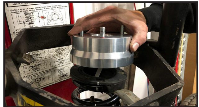
18. Using the strut compressor. Compress the top hat and coil, So the shock stud is coming through the hole in the top hat.
