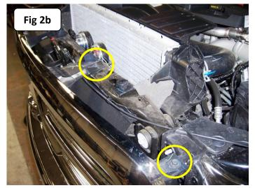
**Step-3** Remove the (2) plastic push in connectors securing the radiator shield to the radiator support using the tip of a screw driver and the bolts (1) per side securing the top of the intercooler to the radiator support using a 13mm socket and ratchet, (Fig 3b).
