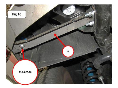
**Step-7** With assistance, adjust and hold the bumper shell visual alignment position, then tighten all supplied nuts and bolts securing all brackets, winch tray and bumper shell.
