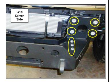
**Step-4** Use a reference point on the vehicle, measure and adjust the winch tray so the side to side alignment on the vehicle is equal, then finger tighten all factory and supplied nuts and bolts securing the winch tray and frame brackets, (Photo 11 & 12).
