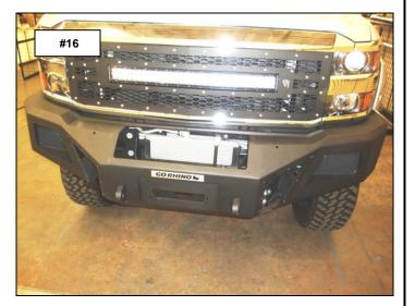
If installing a winch, install the roller fairlead to the bumper shell at this time. Refer to the winch manufacturer's instructions for installation. If installing an optional light bar, install the light bar to the bumper replacement at this time. Refer to the light bar instructions for installation.
