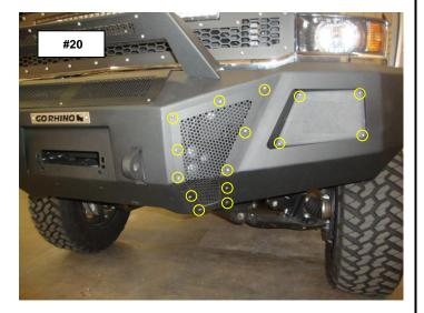
If your state law requires a front license plate, attach the license plate bracket to the holes in the face of the bumper shell, using the supplied 3/8" bolts, washers and nuts, and the license plate to the (2) obround holes in the license plate bracket using the supplied  $\frac{1}{4}$ " bolts and nuts.
