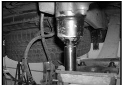
6. Carefully lower down on both hydraulic floor jacks at the same time allowing enough room for the new rear add-aleafs to be installed. Working on the driver side, remove the stock block from the stock location and set aside. Repeat procedure on the passenger side.
