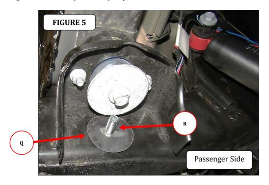
**Step-4** Position the ½" double bolt plate inside the passenger side frame rail, so the (2) bolts extend down through the (2) holes in the bottom of the frame rail, (FIGURE 6).
