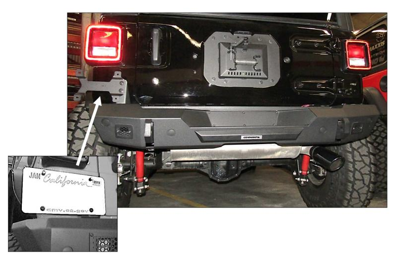
**Step-12** Attach the license plate to the license plate bracket using the supplied ¼" x ¾" button head hex drive bolts, ¼" flat washers, ¼" lock washers and ¼" hex nuts.
