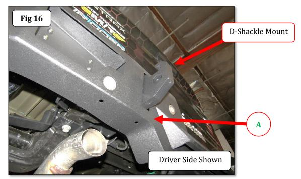
**Step-18** Align the holes and attach the auxiliary brackets to each frame bracket using (2)  $\frac{1}{2}$ " x  $1-\frac{1}{2}$ " carriage bolts, (2)  $\frac{1}{2}$ " flat washers, (2)  $\frac{1}{2}$ " lock washers and (2)  $\frac{1}{2}$ " Hex nuts, (Fig 17). Leave the nuts and bolts loose for final adjustment.
