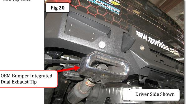
**Step-23** Align the BR20.5 bumper with the vehicle, verify that the tailgate clears the top of the bumper replacement when lowered, then tighten all nuts and bolts.
