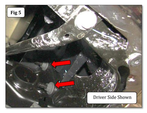
**Step-6** On each side of the vehicle use a 21 mm socket and remove (1) nut securing the outer support bracket to the stud on the side of the frame, (Fig 6).
