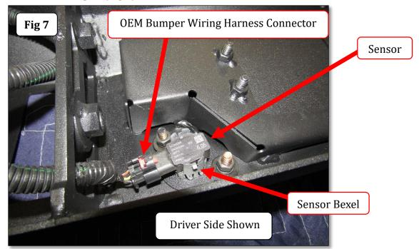
**Step-11** Reconnect the tag lights to their housing (Fig 7) and the OEM bumper wiring harness connector to each Lane Change Alert with Side Blind Zone Alert module, (Fig 9).
