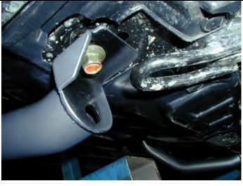
10. Place the large packer (washer) on top of the lower brackets both sides and push the bolt back thru to its original hole, leave these finger tight at this stage.
