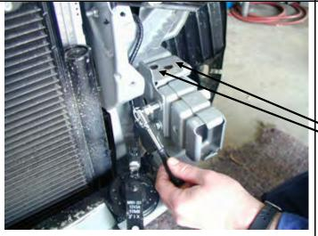
7. Remove the two horns from the left & right hand sides.
