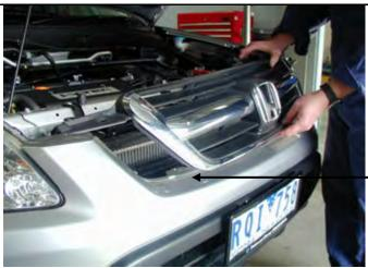
3. The upper radiator cover and the grill must be removed prior to removal of the bumper bar.
