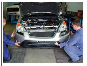
5. With all the fasteners out of the bumper, it is now ready to be removed. If the vehicle is fitted with factory fog lamps, these will need to be disconnected prior to the bumper being removed.
