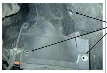
1. The front lower splash guard must be removed from the vehicle, trimmed & re-fitted before the nudge bar can be fitted.
