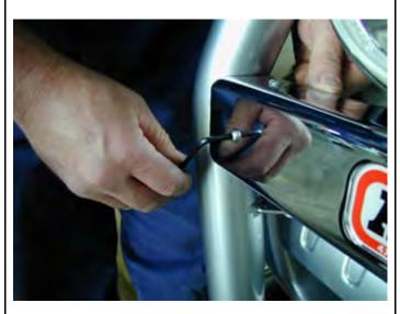
12. Bolt the number plate to the nudge bar using the two M6 button head bolts and flange nuts supplied.
