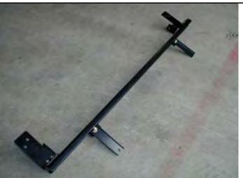
6. Pre-assemble the left hand & right hand chassis brackets to the cross brace using the M8 x 20mm bolts, flat washer and flange nuts.
