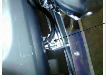
11. Using the M8 x 20 mm bolts, flat washer and flange nuts, bolt the strap type bracket to the nudge bar mounting tabs. You will need to lift the bar up to align the brackets to be bolted.
