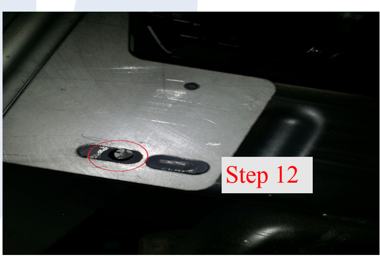
Step 12: Install bracket loosely with bolt tabs
