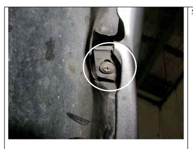
5. Unscrew bumper retaining screws in upper wheel arch area, 1 x screw per side
