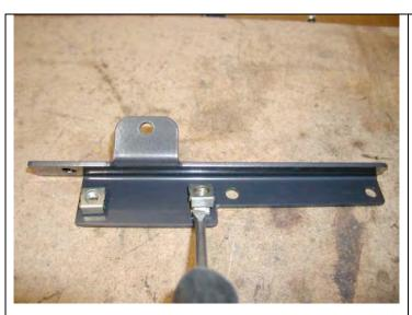
20. Fit M8 cage nuts to brackets as shown, noting that in the bolt kit, there are 4 x cage nuts to suit 3mm mount sheet and 4 off to suit 4mm. These ones are for 3mm and are identified by a shorter clip flange height than the others.
