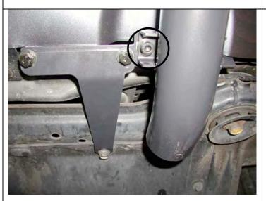
27. Fit M8 cap screw and washer sets to secure lower mount points on nudge bar frame assembly. Take care not to damage paint work on tube with allen key as it is in close proximity to tube when doing up cap screws.
