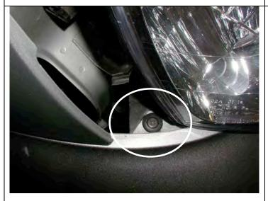
4. *IMPORTANT:* Unscrew plastic retaining screws on bumper tabs under headlight area
