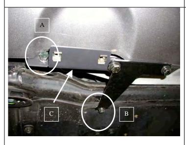
22. Mount bracket assembly each side as shown. An M8 screw washer and nut assembly is used at point 'A'. Note that the *existing* M6 bolt at 'C' is not shown this view, but is fitted through the bracket flange over the plastic bumper tab. The rear mount point 'B' is an existing M8 screw used to secure splash pan.
