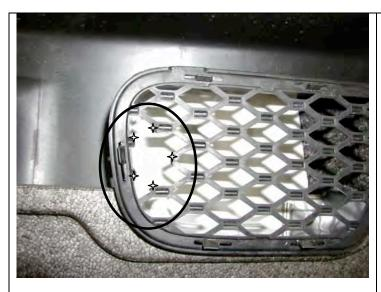
11. Using cutting tool, cut away sections located on outer sides of plastic grill area as shown (circled, stars indicate trim points). This allows mount bracket flanges to fit through the grill area.
