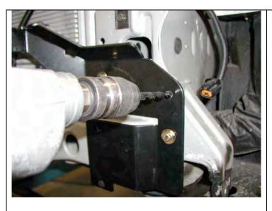
15. Using Dia 9.0 drill, using existing hole as a guide, drill hole through shim and flange. Repeat for other hand.
