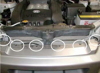
3. Unscrew 6 x plastic retaining screws at top of bumper.
