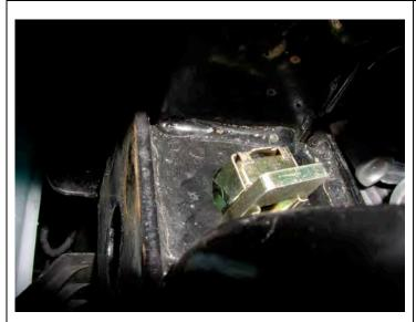
1. Fit M12 caged nut to 3193732 plate. Insert assembly into front hole of chassis member immediately above tow hook as shown. This nut assembly fits between the bars from the tow hook and is used for the M12x40 screw to bolt up bracket assembly.
