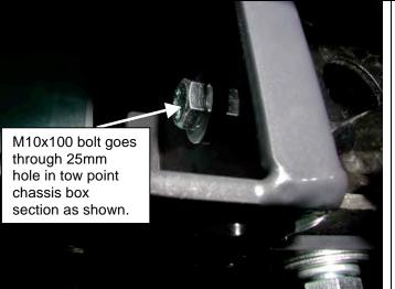
Fit bracket P#3756588 assembly to tow point chassis box section, securing with M12x40 screw, flat and spring washers. Insert M10x100 bolt, 2 x M10 flat washers, large flat washer and M10 nyloc nut as shown. Tension up bolt and screw taking care not to over-tighten the M10 bolt assembly, which could crush the chassis box section.
