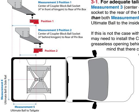
3-1. For adequate tailgate and side rail clearance
