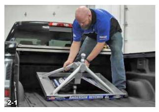
that the coupler tube set bolts are loose enough to allow free movement of the coupler tube.
