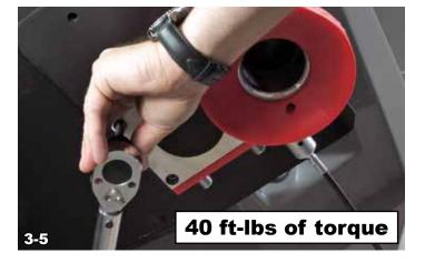
**NOTE:** Because kingpins vary in height, some blocks will have space between the coupler block and the kingpin plate (as shown at right) while others will be flush. This is normal and does not affect performance at all.
