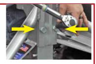
**2-1**. Place the Ultimate Connection base in the bed of your truck with the Ultimate Ball closest to the tailgate. You can use your bed grooves to square up the hitch before tightening it down.
