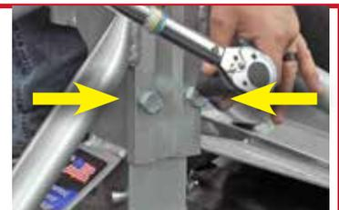
**2-1.** Place the Ultimate Connection base in the bed of your truck with the Ultimate Ball closest to the tailgate. You can use your bed grooves to square up the hitch before tightening it down.
