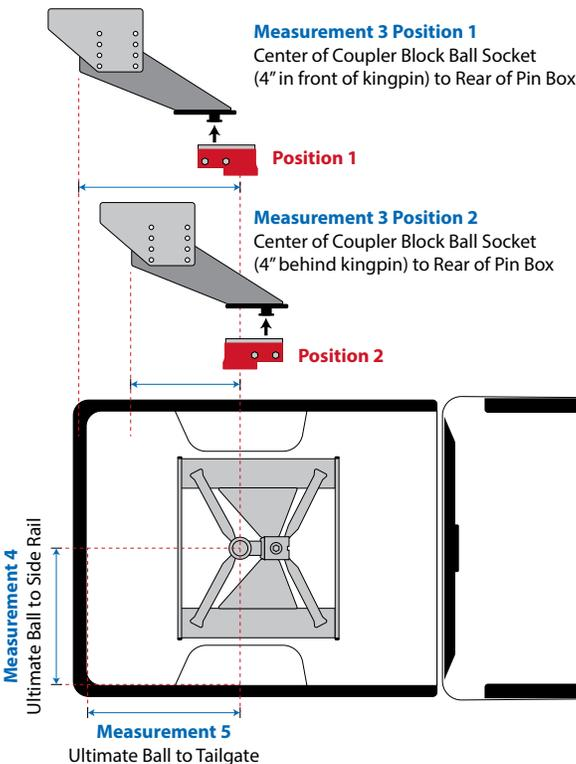
**3-1.** For adequate tailgate and side rail clearance **Measurement 3** (center of the installed Coupler Block's ball socket to the rear of the trailer's pin box) **should be shorter than** both **Measurement 4** and **Measurement 5** (center of the Ultimate Ball to the inside of the side rails and tailgate).
