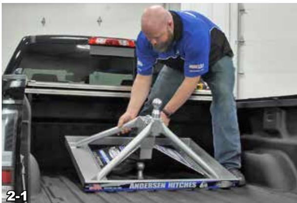
**IMPORTANT** Ensure that the coupler tube set bolts are loose enough to allow free movement of the coupler tube.
