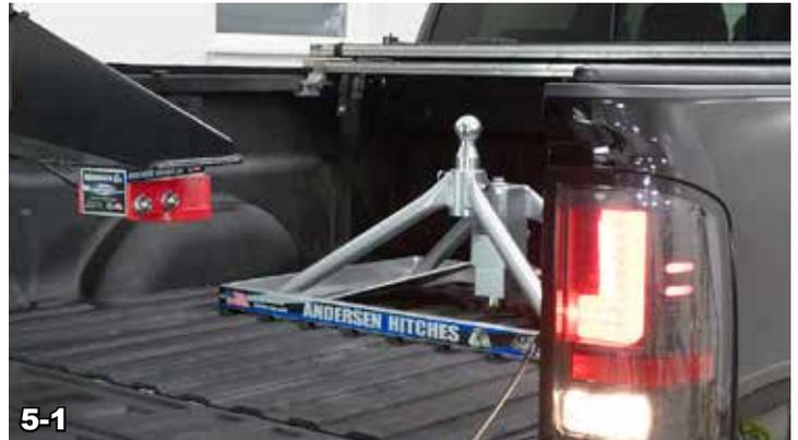
**NOTE:** The red ball funnel that is part of your Kingpin Coupler allows you to easily hook up the Ultimate 5th Wheel Connection, even when up to 3" off center.
