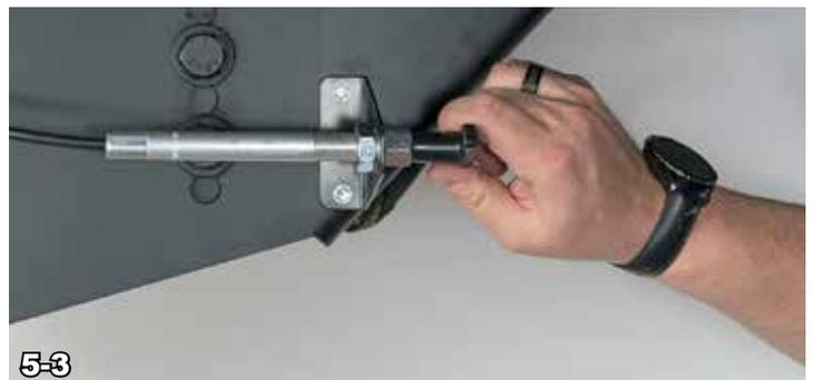
❖ **IMPORTANT** DO NOT FORCE THE LATCH CABLE HANDLE INWARD. If the handle will not push in fully, check to make sure that the receiver is fully seated over the Ultimate Ball.
