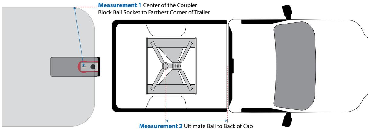
**1-2. If Measurement 1 is SHORTER than Measurement 2 then you might be close to having perfect clearance.** However, "perfect clearance" is not really necessary for 5th wheel trailer towing, most truck/trailer combinations work great with 60°-70° turning clearance. If you want more details about turning clearance, watch the short video clip on our website at the link below (or scan the QR code).
