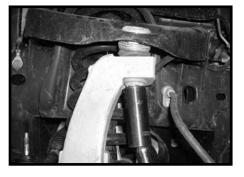
6. Working on the driver side, remove the upper control arm from the knuckle. Let the knuckle hang. Special note: make sure not to over extended any brake hose and or wires.
