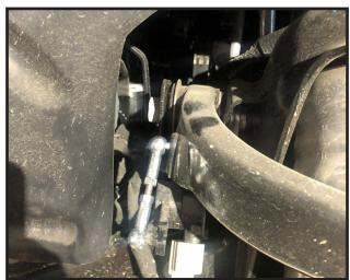
3. Secure the links with the safety clips provided in each end.
