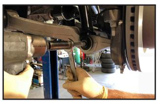
4. Carefully remove the lower control arm mounting/adjusting bolts so that the lower control arm can be dropped out of its frame pockets. Special Note: once these bolts are removed, the lower control arm and front suspension will be able to drop out quite a bit, be careful not to over extend any front brakelines or ABS wires.
