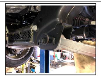
12. Re-install the sway bar endlink lower mount and secure using the OE hardware. Torque to **40 ft lbs.**
