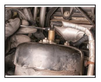
7. Move to the upper strut mounting hardware and remove the 3 nuts. Carefully lower the strut assembly out of the vehicle.
