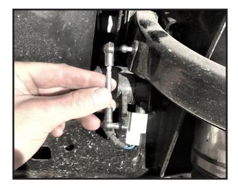
The **safety clips** included are used to lock each ball joint on after installation. They insert from the bottom of each ball joint in the small pin hole then wrap around the neck locking them into place. Please remove locking clips from both ends of the links before installation.
