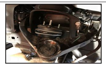
8. Locate a new front strut spacer and install it on the top of the OE strut. Secure the new spacer to the strut using the OE hardware. **Torque to 45 ft lbs**
