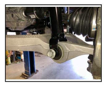
11. Re-install the lower control arm mounting/adjusting bolts and do not tighten yet.
