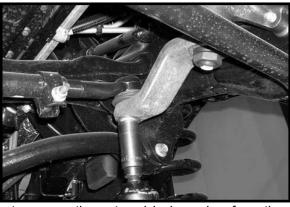
6. Next, remove the nut and lock washer from the sector shaft on the steering box. Save the hardware. Using a pitman arm puller, carefully remove the pitman arm from the sector shaft. The stock pitman arm may be discarded.
