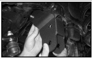
14. Locate the new S10242 sleeve. Also, locate (1) 18 mm x 90 mm bolt, (2) 18 mm flat washers and (1) 18 mm unitorque 17. Install the track bar to the newly installed track bar brackbracket to the stock track bar bracket OE hole. Do not tight-able to install the track bar to the newly installed track en at this point. Special note: The new sleeve will be bar bracket, this step will need to be performed when installed inside the OE bracket.
