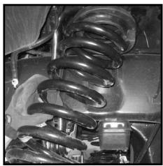
and secure using the new 3/8" hardware. Make sure to add Repeat procedure on the passenger side. loctite and torque to 28 ft lbs. Hole already provided. Special note: When installing the new spacer into the vehicle, make sure that the fat side of the taper goes towards the outside of the vehicle. Also, there is a notch in the upper ring of the spacer also needs to be installed with the notch facing the outside of the vehicle. Repeat procedure on the passenger side.
