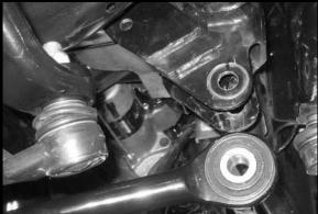
12. Working on the front portion of the OE track bar bracket, carefully enlarge the 3/8" hole to a 1/2" hole using a electric drill.
