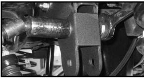
nut from hardware bag 33118NB. Using the new 18 mm bolt, et and secure using the OE hardware. Make sure to use lochardware and sleeve, secure the new track bar relocation tite and torque to 145 ft lbs. Special note: If you are not the suspension system is completely installed and the weight of the vehicle is on the ground.
