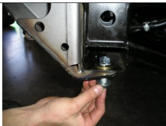
9. Secure lower fixing point by passing through lower bracket in a upward motion, using M12 bolt, 12mm flat washer and secure from the top using large gold coloured 12mm flat washer,12mm spring washer and 12mm nut (fine thread) to each side of vehicle. When all bolts are fitted, tighten securely.
