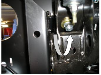
8. Secure from underneath using large 12mm gold coloured flat washer,12mm spring washer and 12mm nut to both sides of vehicle.
