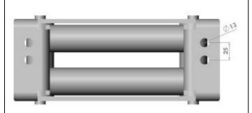
24. Drill two new 13mm holes in the roller fairlead provided in the kit, as shown on the adjacent picture.
