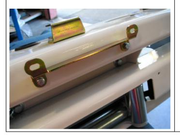
30. Fit number plate bracket to bar using 6mm hardware.
