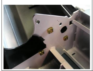
13. Fit M10 caged nuts to the inside of mounting surface of bull bar.
