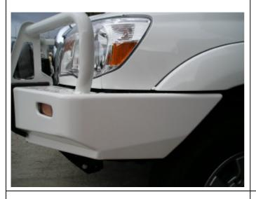
35. Align bull bar so there is a 15mm to 20mm gap around periphery under front vehicle panels, then tighten all bolts securely.
