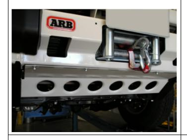
38. Fit splash pan to lower flange of bull bar using M6 x 20mm bolts,6mm spring washers and 6mm large flat washers. Finger tighten only.
