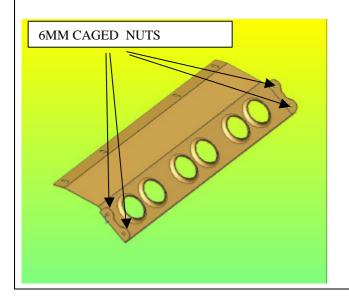
37. Fit M6 caged nuts to the inside of the flanges on the splash pan.
