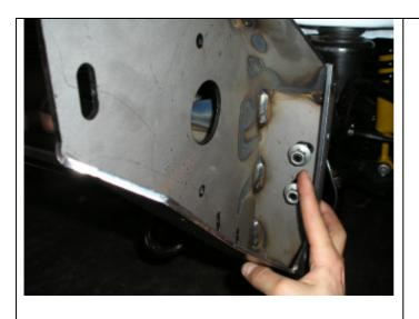
5. Fit original 10mm nuts to the outside fixing points . **See Photo:**
