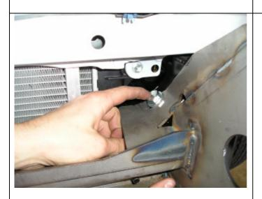
7. Fit 12 x 35mm x 1.25 (fine thread) bolt,12mm flat washer through top rearward bracket passing through body mount.
