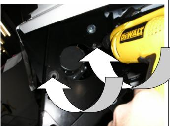
36. Finally, using the existing 2 holes as a template. Drill through using a M10 drill bit and secure using the balance of the 10mm hardware.
