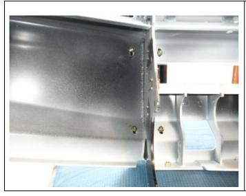
18. Fit buffers to bar and secure from inside of bull bar using 6mm flange nuts. Six to each side of vehicle.
