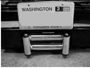
Fitting with winch, number plate above RFL
