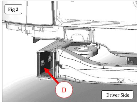
**Note:** It is recommended to apply a strip of duct tape to hold the nut plate in place inside the frame rail prior to positioning the Rockline rear bumper on the frame rails and installing the bolts.
