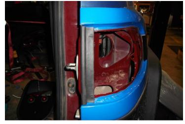
unable to recover it. Each tail light is attached with three carriage bolts which are passed through mounting slots in the tail light housing (Two next to the rectangular LED lights, and one on the side of the housing.) It may be useful to have a helper at this point to help hold things in place outside the vehicle while attaching hardware inside the vehicle.
