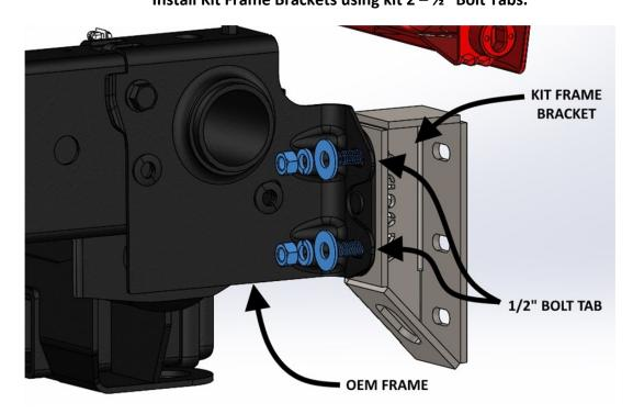
Install kit 3 - ½" Bolt Tabs into each End Pod Bumper Bracket with ½" Retainer Washers. (against bumper)
