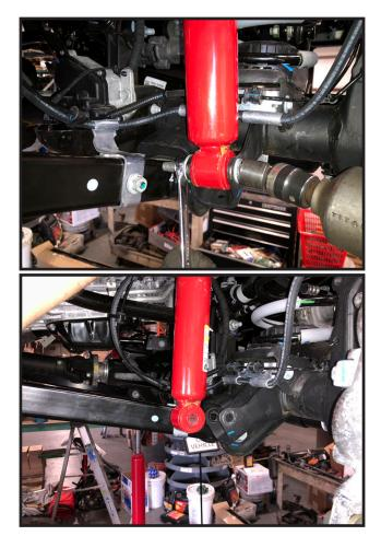
4. Working on both sides, remove the brakeline frame mounting bracket bolt and save bolts.
