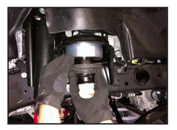
13. Re-install the front coil springs making sure to install them on the same side they were removed from. Also make sure that the bottom of the coils are properly seated in the lower plastic mount so that the end of the coil wind is up against its stop.
