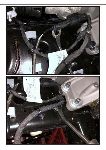
7. Working on the passenger side upper control arm axle mount, locate and remove the plastic wire harness plug from the control arm to gain slack in the wire.
