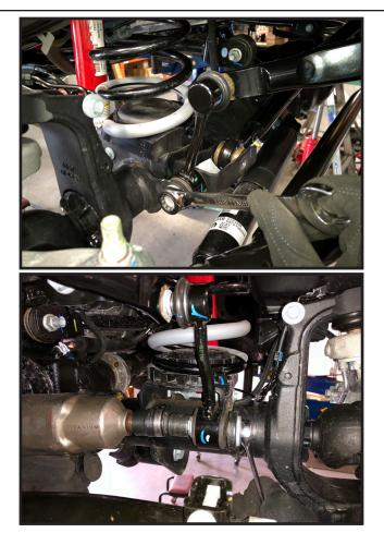
6. Working on the driver side inner frame rail, just behind the steering gear box, locate and remove the plastic plugs holding the wire harness to the frame. This is done to gain slack in the wires during the install process.
