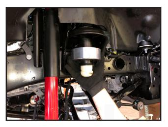
12. Re-install the rubber coil spring isolators to the bottom of the new coil spring spacers.
