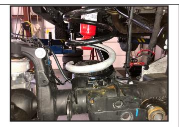
14. Locate the shock Extension Brackets, (2) S10026 Sleeves, (2) 123B, (4) 716WA, (2) 12UN, And the OE shock hardware. Install the bracket on to the lower Shock mount, Using the OE hardware and S10026 sleeve. Do not tighten. Attach the shock to the bracket using 123B, 716WA, 12UN. Do not tighten.
