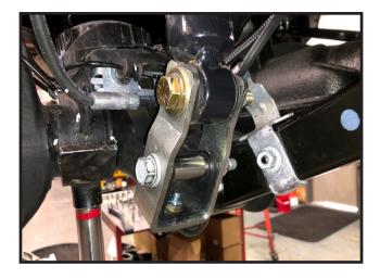
17. Carefully raise up on the hydraulic floor jacks enough to start re-installing all of the previously removed components. **Tip: Place a jackstand or support device under the rear bumper before raising the front axle to help prevent the vehicle from lifting from the pressure of the coil springs.**
