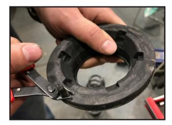
11. Locate the new front coil spacers part #42105-02, and install them into the front coil spring frame mounts.
