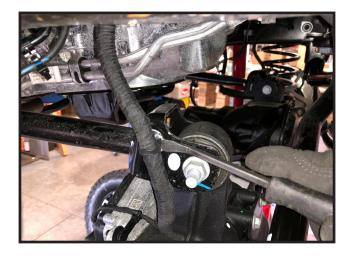
8. Carefully lower down on the hydraulic jacks so that the coil springs become loose and can be removed. Remove the front coil springs and set aside. **IMPORTANT: Be sure to remember what side of the vehicle the coils came off of, they will need to be re-installed on the SAME side as the came off.**
