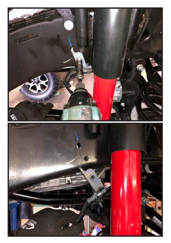
5. Working on both sides, remove the lower mounting hardware for the swaybar endlinks. Save the hardware.
