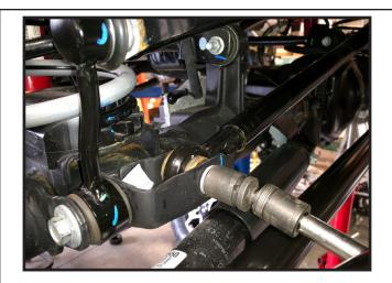
3. Working on both sides, remove the shocks from the axle, save the hardware for later installation.
