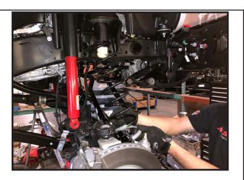
Working on both sides, remove the upper rubber coil spring isolator from the frame mount.
