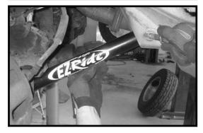
14. Locate the new track bar relocation bracket. Install the new bracket into the OE track bar pocket.
