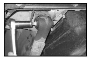
38. Locate the new rear springs. Remove the bushings and sleeves from the new springs and add some lithium or moly base grease to the bushings and sleeves and re-install them back into the new springs. This will help prevent squeaking the life of the bushings and will also improve ride quality.
