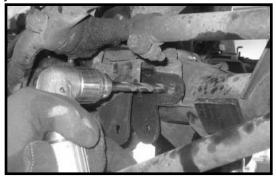
17. Locate (1) 3/8" x 1" bolt, (2) 5/16" USS flat washers and (1) 3/8" unitorque nut from hardware bag 43800NB. Secure torque to **18 ft lbs.** Repeat procedure on the passenger side. the new track bar bracket to the OE bracket using the new 3/8" hardware. Make sure to use loctite and torque to 32 ft lbs.
