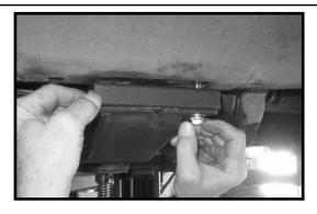
installed transfer case spacer hardware and torque to 28 ft OE location. The u-bolts and hardware may be discarded. Ibs. Repeat procedure on the passenger side. Carefully The upper u-bolt plate can rest on top of the spring. Repeat remove the hydraulic floor jack from under the transfer case procedure on the passenger side. cross member.
