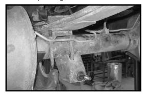
35. Remove the rear brake line from the OE brake line bracket.
