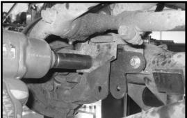
19. Locate (1) 10 mm x 70 mm bolt, (2) 5/16 USS flat washers and (1) 10 mm unitorque nut from hardware bag 43800NB. Install the track bar to the newly installed bracket and secure using the new 10 mm x 70 mm bolt and hardware. Make sure to use loctite and torque to 28 ft lbs. Special note: If you are not able to install the track bar to
