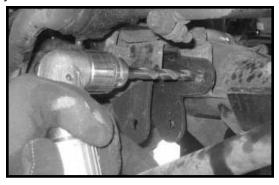
(1) 3/8" unitorque nut from hardware bag 43800NB. Secure senger side. the new track bar bracket to the OE bracket using the new 3/8" hardware. Make sure to use loctite and torque to 32 ft 20. Working on the driver side, secure the new brake line lbs.
