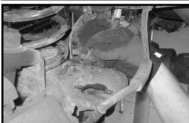
Carefully lower down on both hydraulic floor jacks at the same time allowing enough room for the OE coil springs to be removed. Remove the OE coil spring and discard. Repeat
