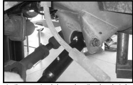
11. Locate the new EZ-Flex control arms. Set each control 13. Locate the new track bar relocation bracket. Install the new bracket into the OE track bar pocket.
