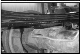
39. Locate the proper u-bolts. Also, locate (8) 1/2" u-bolt washers and (8) 1/2" high nuts from hardware bag 12NW Working on the driver side, install the u-bolts into the OE location and secure using the new hardware. Torque to 85 ft **Ibs.** Repeat procedure on the passenger side.
