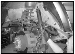
Working on the driver side, remove the sway bar endlink from the sway bar and axle location. Save the hardware and endlink. Repeat procedure on the passenger side
