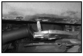
29. Locate the new transfer case cross member. Locate (4) 10 mm x 50 mm bolts, (4) 3/8" lock washers and (4) 3/8" SAE washers from hardware bag 43800NB. Working on the driver side, install the new transfer case spacers between the cross member and the frame. Secure using the new hardware. **Do not tighten at this point.** Repeat procedure on the passenger side.
