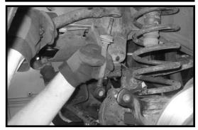
4. Working on the driver side, remove the brake line bracket
