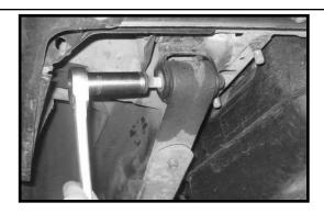
Locate the new rear springs. Remove the bushings and sleeves from the new springs and add some lithium or moly base grease to the bushings and sleeves and re-install them back into the new springs. This will help prevent squeaking, the life of the bushings and will also improve ride quality.
