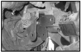
15. Make sure that newly installed track bar bracket is seating flush in the OE pocket. Using the new bracket as a guide, 18. Locate (1) 10 mm x 70 mm bolt, (2) 5/16 USS flat washcarefully drill a 3/8" hole into the OE bracket.
