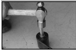
38. Working on the driver side, install the new rear spring of the vehicle is on the ground. Repeat procedure on the the new clevis mount into the upper end of the rear shocks.
