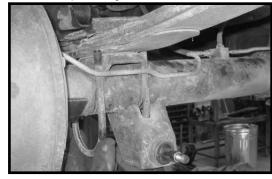
34. Remove the rear brake line from the OE brake line bracket.
