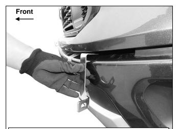
(Fig 10) Carefully insert bent end of Driver/Left Support Bracket through gap between lower bumper and upper plastic fascia panel. Use removable tape to protect finish on bumper
