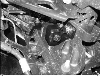
(Fig 12) Driver/left Mounting Brackets installed, pictured from behind/below bumper
