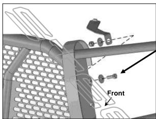
(Fig 19) Attach 2014-on driver/left Top Bracket to upper hole in Grille Guard
