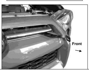
(Fig 14) 2014-on, driver/left Top Bracket installed
