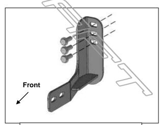
(Fig 4) Reuse the factory bolts to attach driver/left Frame Bracket to front of bumper bracket
