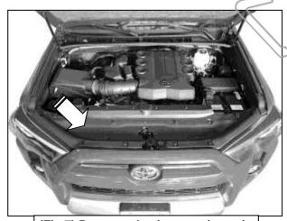
(Fig 7) Remove plastic cover (arrow)
