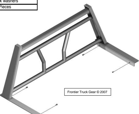
**Step 1:** Position and center headache rack on truck bed allow for space between rack and cab of truck.
