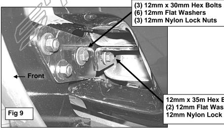
12mm x 35m Hex Bolt (2) 12mm Flat Washer 12mm Nylon Lock Nut
