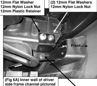
12mm x 35m Hex Bolt (2) 12mm Flat Washer 12mm Nylon Lock Nut
