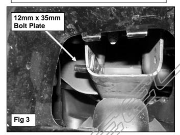
12mm x 35mm Bolt Plate 12mm Flat Washer 12mm Nylon Lock Nut 12mm Plastic Retainer
