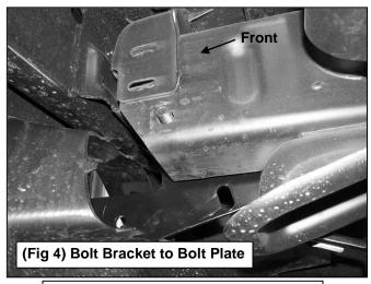
Inner wall of passenger side frame channel pictured from behind bumper
