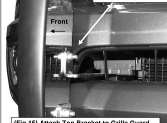
(Fig 15) Attach Top Bracket to Grille Guard
