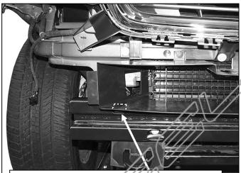
(Fig 4) Hold Top Bracket in place to determine area to cut from air deflector
