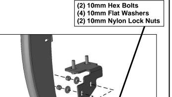
(Fig 13) Attach Grille Guard to outside of driver/left Frame Bracket
