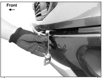
(Fig 10) Carefully insert bent end of driver/left Top Bracket through gap between lower bumper and upper plastic fascia panel. Use removable tape to protect finish on bumper
