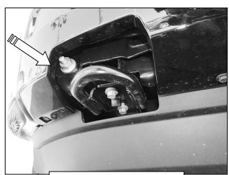
(Fig 2) Remove plastic cover surrounding tow hook
