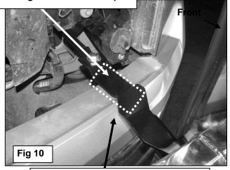
Protect the top of the plastic bumper cover with masking tape to prevent scratches during installation
