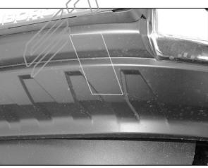
(Fig 15) Cut area pictured for example only. Installer responsible for correct modifications
