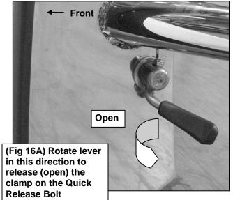
To open the hood, release the lever on the Quick Release Bolts. Try to pull the Grille Guard forward. If Necessary, loosen the Hex Bolts securing the Grille Guard to the Mounting Brackets. Only loosen the hardware enough to move the Grille Guard
