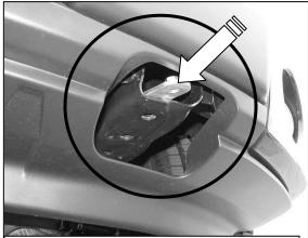
(Fig 2A) Insert Nut Plate through opening in end of frame (NOTE: Tow hook model pictured for instruction purposes only)
