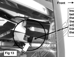
Insert a 3/8" Plastic Washer between the Grille Guard and the slotted Top Bracket. Line up the hole in the Plastic Washer with the mounting holes. Insert the Quick Release Bolt through the Plastic Washers
