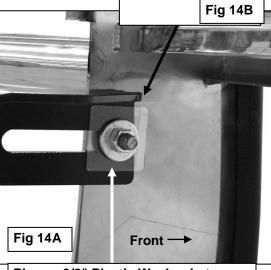
Place a 3/8" Plastic Washer between the slotted Top Bracket and the 3/8" Flat Washer to protect the finish on the Top Support Bracket
