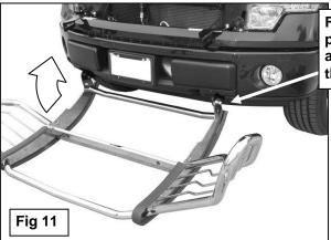
For easier installation, insert (1) 12mm Hex Bolt per side in the location pictured in Figure 8 to act as a hinge. Snug the hardware but do not tighten, then rotate the Grille Guard up into position
