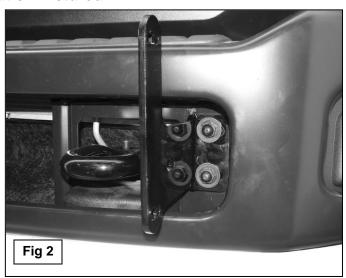
**WARNING!** Do not remove passenger and driver bumper bolts at the same time or bumper may fall. Only remove and install one Frame Mounting Bracket at a time.
