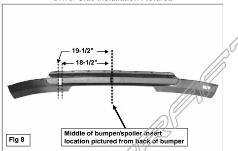
Draw lines to represent the top and the bottom of the Frame Bracket
