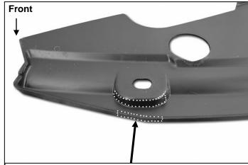
(Fig 15) Driver side-bottom of plastic cover pictured. Cut out area as indicated by dotted line
