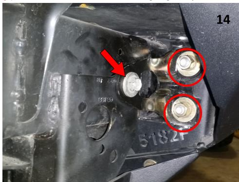
15 Once all the bolts are installed and bumper is properly adjusted; tighten all bolts at this time.
