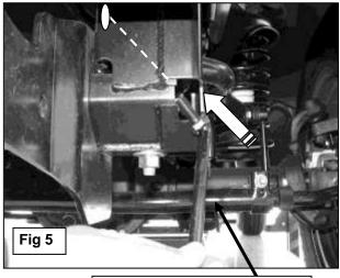
Insert (1) 8mm Rod Bolt up through opening in corner, hole in Top Bracket and out hole in side of frame upright
