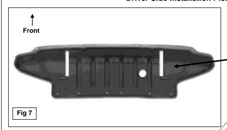
**Once the Mounting Brackets have** been installed and checked for alignment, hold the splash guard up into position and mark the cut area on the inside of the guard. Start with a small opening and slowly enlarge the opening to get the best fit around the brackets. Area cut from guard pictured for example only. (Interior view)
