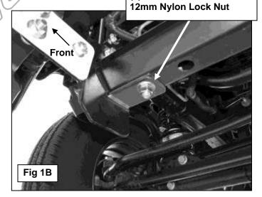
2010-12 Passenger side Frame Mounting Bracket bolts to the inner mounting location (pictured with Grille Guard in position for example only)
