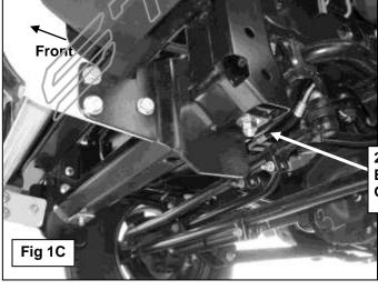
2007-12 Driver side Frame Mounting Bracket installation (pictured with Grille Guard in position for example only)
