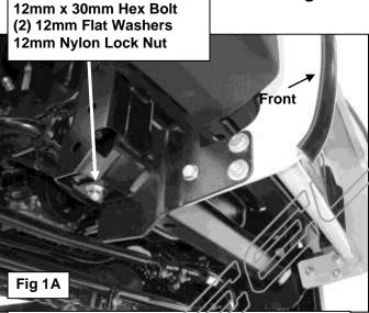
07-09 Passenger side Frame Mounting Bracket bolts to the outer mounting location (pictured with Grille Guard in position for example only)
