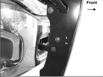
(Fig 14) Attach Grill Guard to outside of Mounting Brackets (passenger/right side pictured
