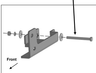
(Fig 9) Attach driver/left Frame Bracket to tow hook and forward tow hook mounting hole (Fig 8)
