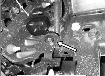
(Fig 10) Remove hex bolt (arrow)
