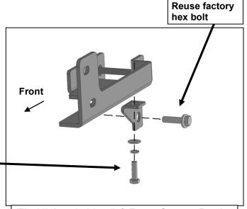
(Fig 11) Attach driver/left Frame Support Bracket to side of frame and bottom of Frame Bracket
