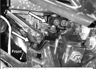
(Fig 6) Driver/left Top Bracket and Top Support Bracket pictured from behind bumper
