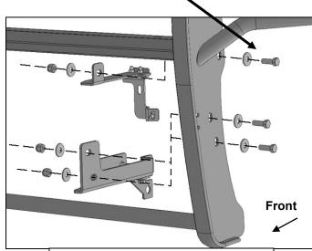
(Fig 13) Attach Grill Guard to outside of driver/left Mounting Brackets
