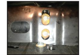
NOTE: If vehicle has a side-lean, install the 10mm spacer supplied in kit. In our experience, the driver side is most often the low side.
